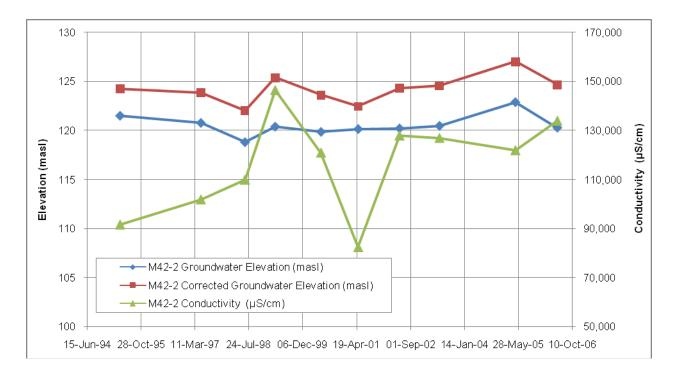
For this dataset, representative of extremely saline groundwater, the correction to measured pressure head values is on the order of 2 to 4 m.
