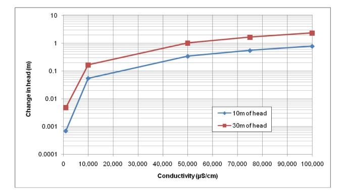
Electrical conductivities measured at groundwater monitors at the WM Richmond site exhibit an extremely large range of values from hundreds of  $\mu$ S/cm to over 100,000  $\mu$ S/cm at some locations. This is illustrated below for two on-site monitors: M42-2 (a deep bedrock monitor with saline groundwater and very high electrical conductivity) and OW4 (a shallow bedrock monitor with fresher groundwater conditions and moderate conductivity).
