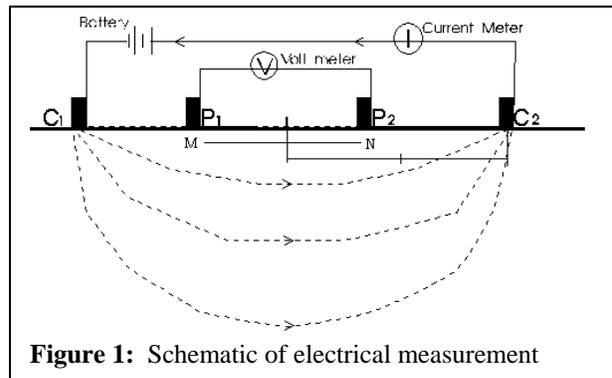
Figure 1: Schematic of electrical measurement
