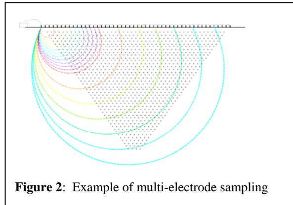
During Phase 1A, both 2.5 and 5 metre electrode spacings were tested. It was determined that the 2.5 metre spacing provided adequate penetration and resolution and this spacing was, therefore,
