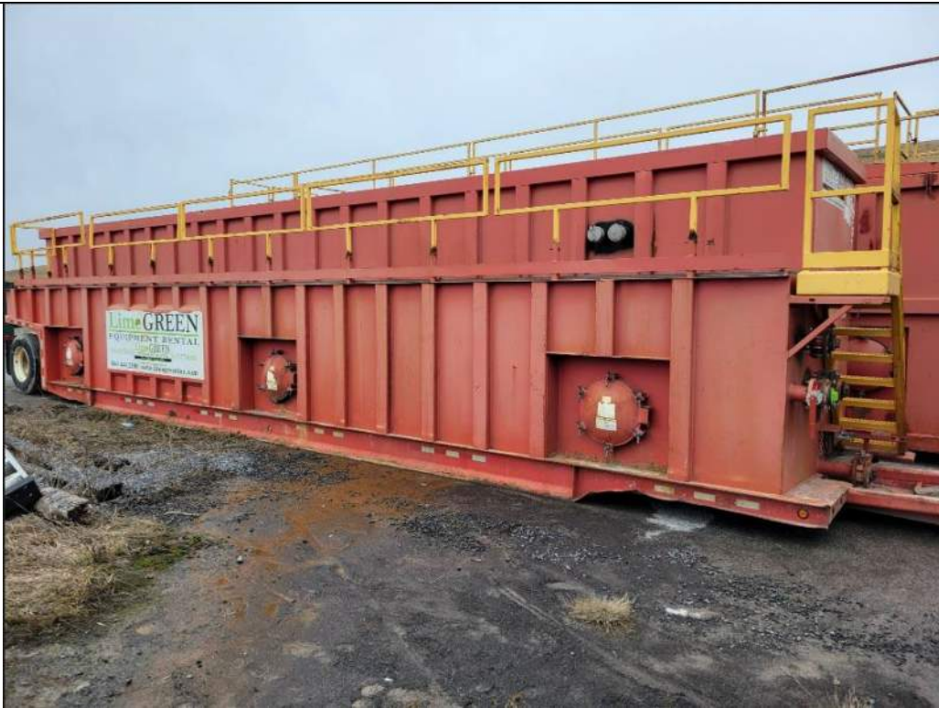
Photograph 1 (March 27, 2023). Frac tank showing evidence of leakage (rust coloured staining on ground).
